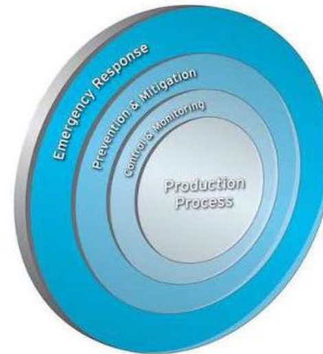
Figure 1: IEC 61511 prescribes separate safety layers from control and monitoring, prevention and containment, as well as emergency measures. Image courtesy: Control Engineering Europe/Hima
